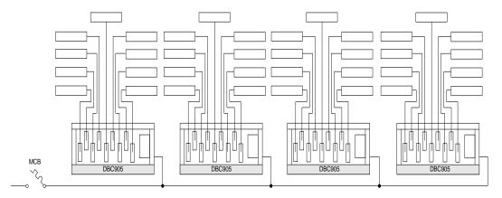
The DBC905 can also support multiple light fixtures connected to a single output to deliver greater economy if required. Care again should be exercised with this approach to not exceed output capacity limitations. It should be noted that each group of three output channels (CH1,2,3, CH4,5,6, CH7,8,9) is protected by a replaceable slow blow 6.3A HRC fuse.
