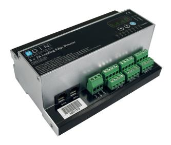
An eight circuit dimmer module rated at 500W per circuit for the control of resistive and inductive lighting loads with the facility to select dimming or switched only operation of any circuit. A custom designed housing provides reliable power handling in a compact format.
