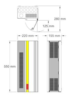
SCH1210 D version - 690x220x155mm. RCBO & RCBOX version - 550x255x155mm
