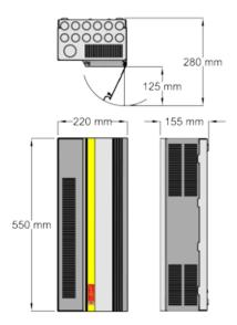
SCI1205 D version - 690x220x155mm. RCBO & RCBOX version - 550x255x155mm.
