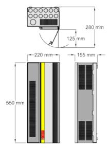
SCLED1205 D version - 690x220x155mm. RCBO & RCBOX version - 550x255x155mm.
