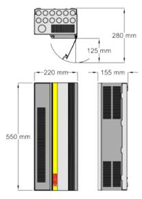
SCS1210 D version - 690x220x155mm. RCBO & RCBOX version - 550x255x155mm
