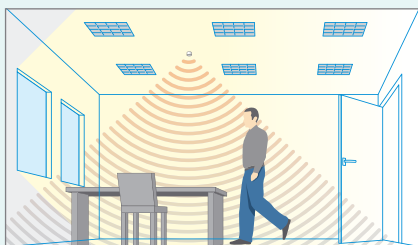
Presence detected, sufficient daylight, lights off.
