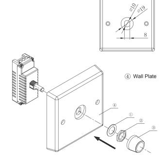
3.7.3 Carefully position all wires inside the junction box, leaving enough room to insert the dimmer housing. Put the dimmer into the junction box and fix it using screws.
