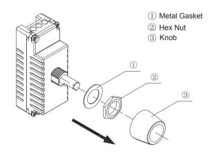
3.7.2 Fix the dimmer on the wall plate, then fix the metal gasket and hex nut orderly on the wall plate, install the knob finally, gently push it to ensure flush fit.
