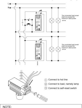
One push button switch can control up to 20pcs of dimmer for UP/DOWN dim and ON/OFF at the same time.
