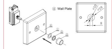
3.7.3 Carefully position all wires inside the junction box, leaving enough room to insert the dimmer housing. Put the dimmer into the junction box and fix it using screws.
