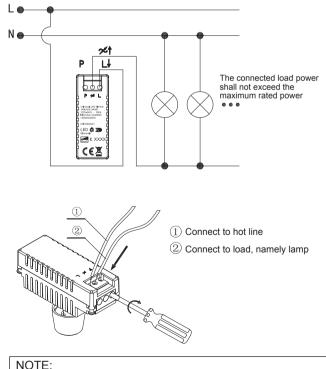
Two or more dimmers must not be connected in parallel or series to control the same load from two different locations.
