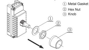
3.7.2 Fix the dimmer on the Wall Plate, then fix the metal gasket and hex nut orderly on the Wall Plate, install the knob finally, gently push it to ensure flush fit.
