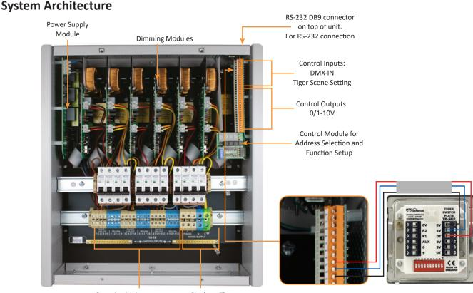
Outgoing Mains Circuit Connections Single or Three Phase Mains Input
