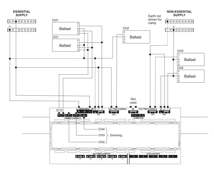
As shown in the above diagram, the unit may also be wired with two different supplies where one of the supplies is guaranteed to be available referred to as essential, while the other is referred as non-essential supply. The unit is recommended to be powered using the essential supply. As shown in the diagram, one or more channels may be powered from either of the supplies.
