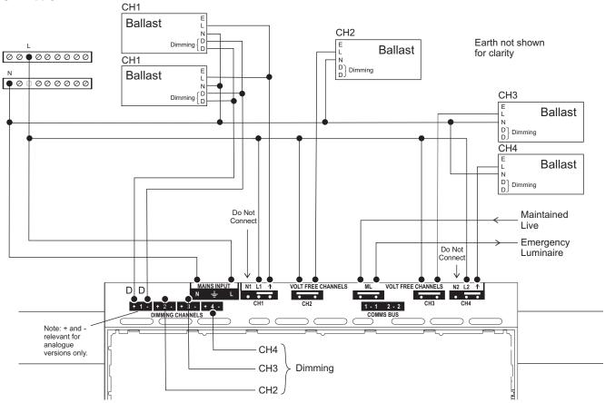
As shown above, the unit can be powered from a single supply; one or more luminaires may be connected to each channel.
