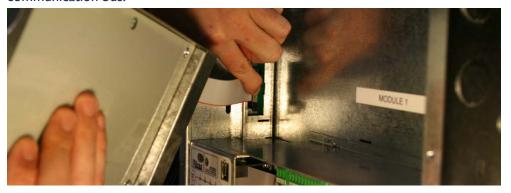
3. Locate the tab and slide the module into position.
