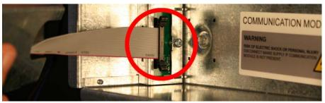
3. Align the mounting tab with the slot on the left and slide the module into position.
