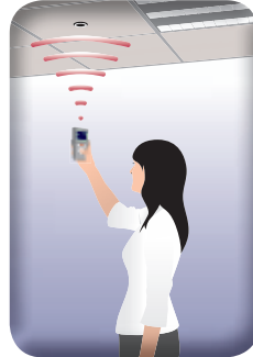
Upload settings to detector - the luminaire blinks to confirm
